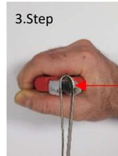
Attention! When bending, make sure that the eyelet does not exceed 6mm to ensure good contact with the anode rod.
